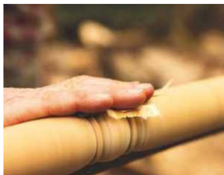
An interesting trick. A handful of shavings is used to burnish and smooth the finished piece
